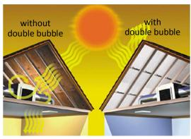
Double bubble will help reduce downward radiant heat flow and help prevent condensation from building up on the interior metal roof surface. Reduce peak summer attic temperatures by up to 40 deg. F with double bubble radiant barrier insulation along with proper ventilation from eve vents and gable vents.
